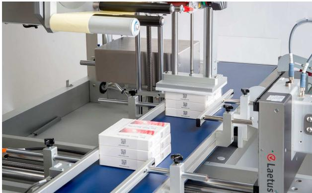
IMV-370 pack handling system for the inspection of bundles
