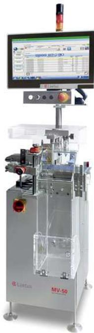
Serialization of folding boxes with the compact pack handling system MV-50.
