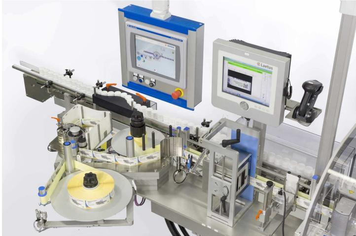
The HERMA 132M all-round labeling system with integrated Laetus Secure Track & Trace Solutions (S-TTS) software.
